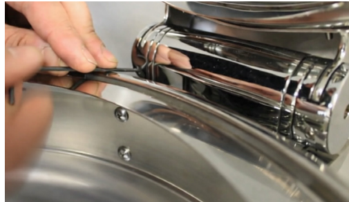
Figure 2: Unscrewing Radiance Induction Buffet Server axle screws at the base of the axle
