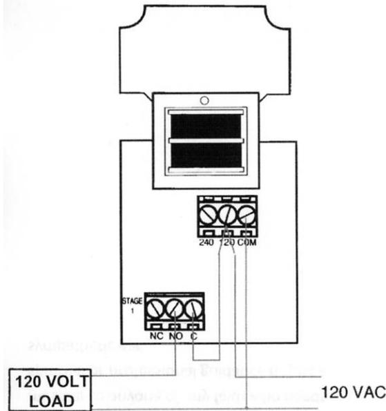
Figure 4: Typical Line Voltage Wiring Diagram.
