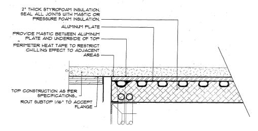
1. ROUT 1/16 "DEEP RECESS ALONG ENTIRE PERIMETER TO ALLOW FOR FLANGE CLEARANCE
