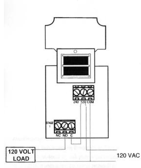
Figure 4: Typical Line Voltage Wiring Diagram.
