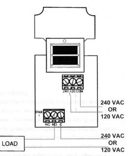
Figure 6: Different Voltage to Control and Different Voltage Load.
