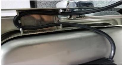
**Figure 3. Electric Heating Element Cord in Holder**
